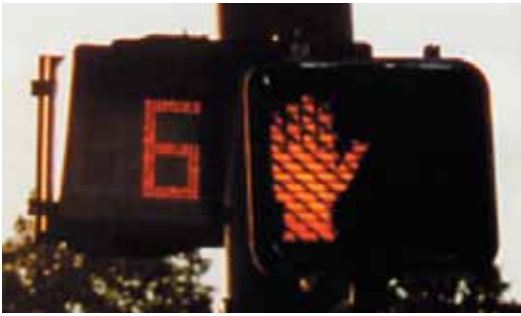
Countdown signals help pedestrians know how much time they have left to cross an intersection.
